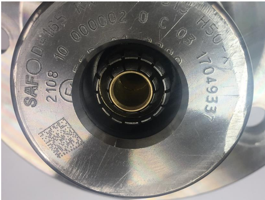
Drilled kingpin top view with Aucos connector inside.
